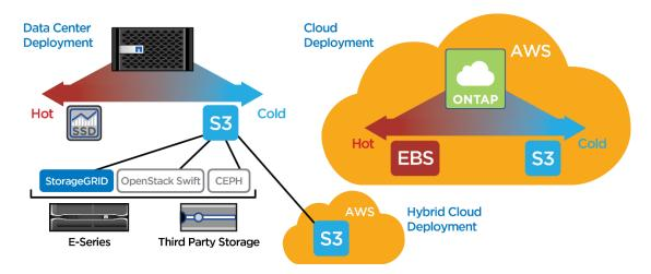
Figure 4) With Fabric Pool, the Data Fabric can intelligently and automatically move data to the optimal tier, whether it be SSD or object media.
