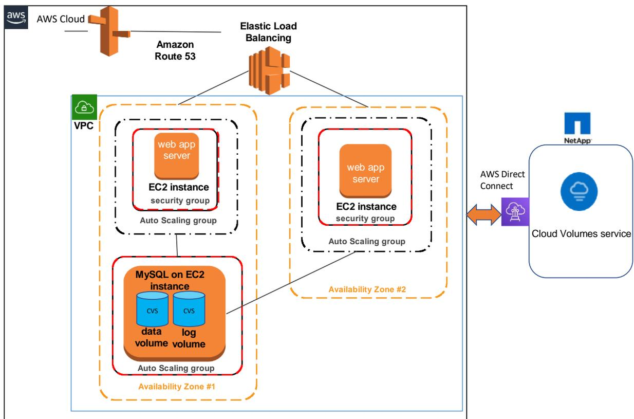
In the architecture diagram, you can see that the MySQL database database volume and log volumes are configured on Cloud Volumes Service for AWS. With the combination of backups, snapshot copies, and right-sized throughput, you can easily host your high-performance database in the cloud with maximum data protection and eight 9s of data durability (soon to be nine 9s).
